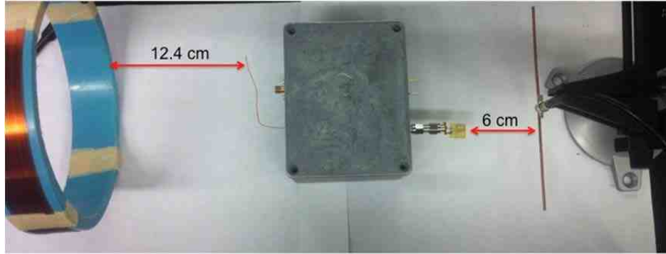
Figure 156. Test setup to determine powering and sensing range.
