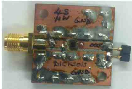
Figure 107. Rectifier circuit 50 \Omega Test fixture.
