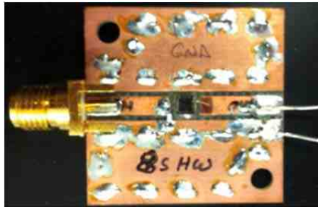
Figure 112. Rectifier 50 \Omega test fixture.
