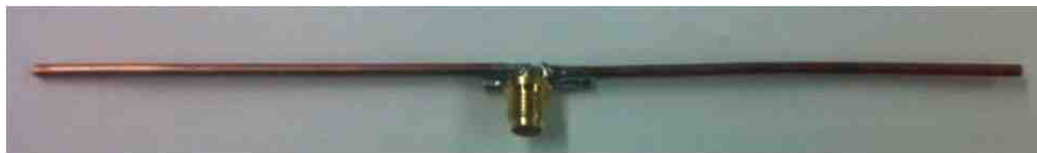
Figure 38. 915MHz half-wavelength wire dipole antenna.
